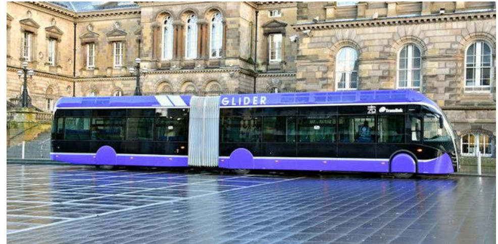
Belfast Glider service - using 18 metre long, articulated vehicles with 105 people capacity
